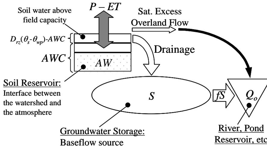
**Figure 2.** Schematic of a daily soil-water and watershed budget.  $D_{rz}$  is root zone depth.
