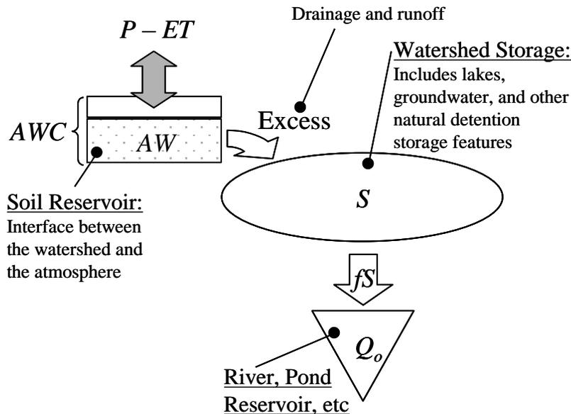
**Figure 1.** The soil reservoir and how it connects to stream discharge at the watershed outlet,  $Q_o$ .
