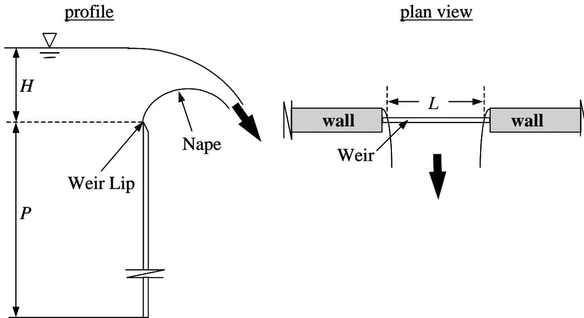
**Figure 1:** Schematic of a sharp crested weir profile and plan view; note that free outfall is shown.
