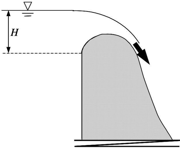
**Figure C.1:** Schematic of the lip of an ogee spillway
