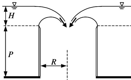
**Figure D.1:** schematic of converging weir flows.
