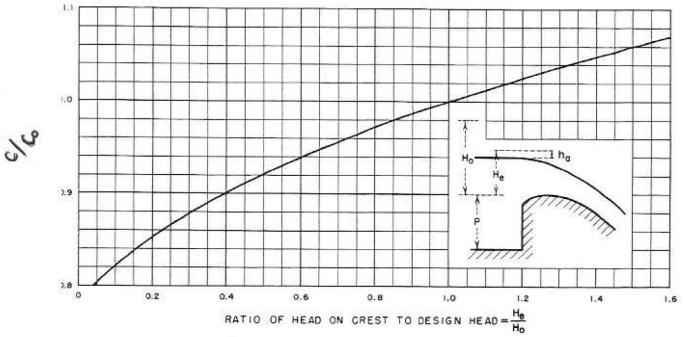
Figure 9-24.—Discharge coefficients for other than the design head. 288-D-2410.
