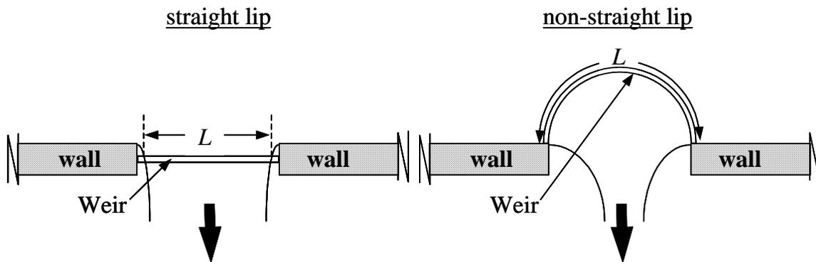
**Figure B.1:** Schematic of a straight and non-straight weir lips in plan view.
