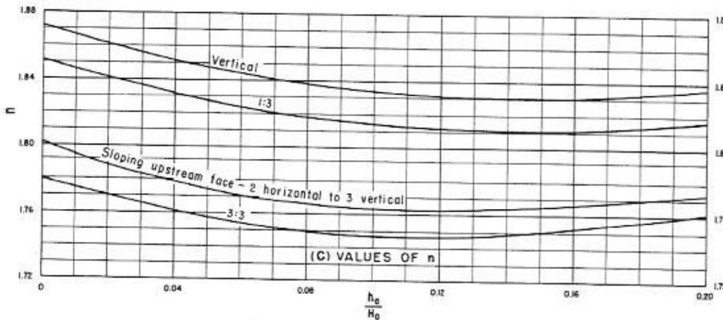
Figure 9-21.—Factors for definition of nappe-shaped crest profiles. 288-D-2406. (Sheet 1 of 2).
