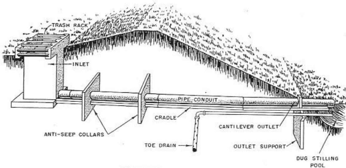
DROP INLET SPILLWAY
