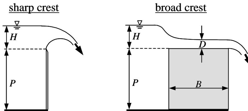
**Figure A.1:** Schematic of a sharp and broad crested weir profiles.
