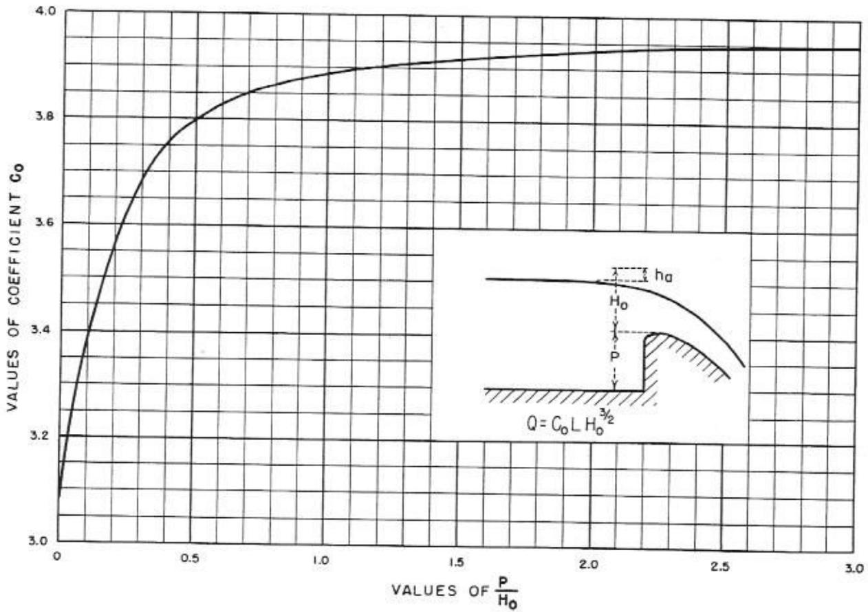
Figure 9-23.—Discharge coefficients for vertical-faced ogee crest. 288-D-2409.
