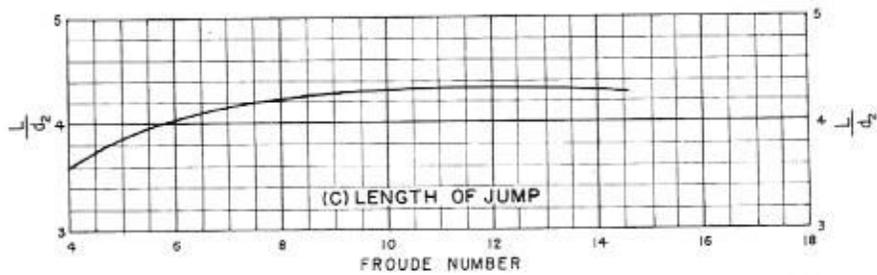
Figure 9-42.—Stilling basin characteristics for Froude numbers above 4.5.
