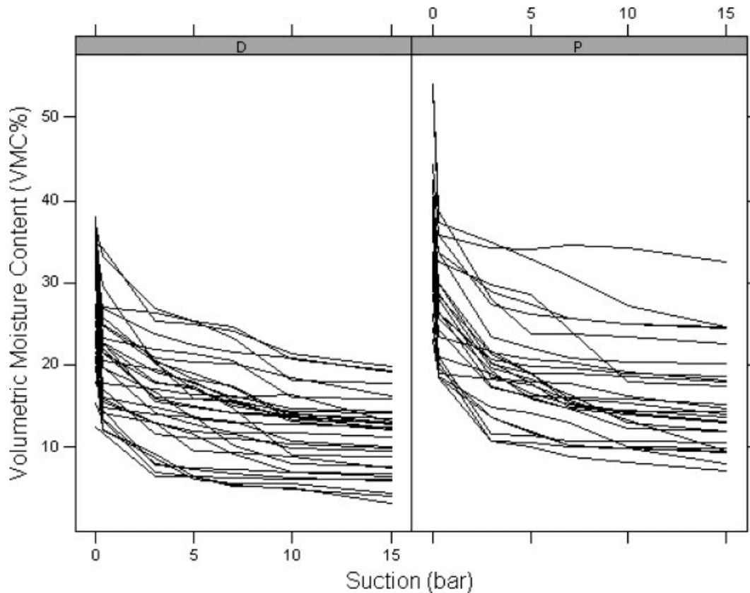
Figure 7. Soil moisture characteristics for 58 samples D = degraded ( $n = 32$ ); P = protected ( $n = 26$ ).
